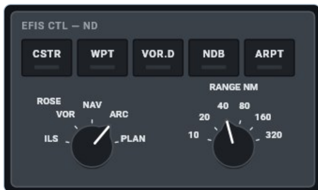
EFIS control panel (ND part).
