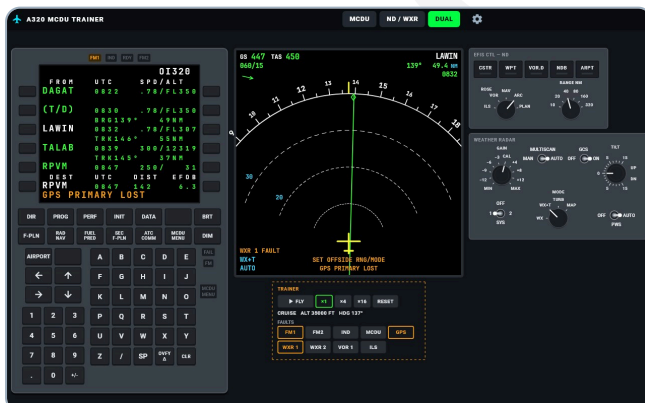
FM1 + GPS + WXR 1 faults.
